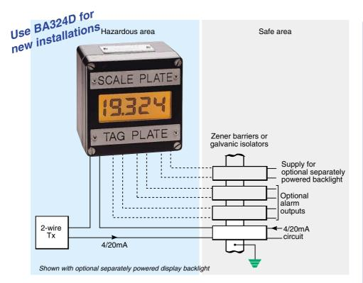
The BA324C is an intrinsically safe field mounting indicator which displays the current flowing in a 4/20mA loop in meaningful engineering units. The indicator has a 20mm high, easy to read liquid crystal display, and is housed in a robust IP66 enclosure. Modular accessories enable only the required features to be incorporated thus reducing cost while retaining interchangeability between instruments.
